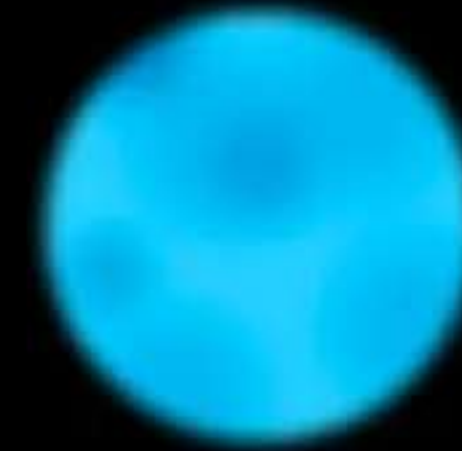
Ordinary Curing Light: Non-uniform light output
